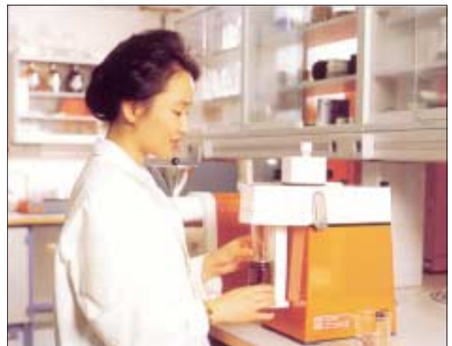
Cyclotec filled with holder for 500 ml sample bottle
